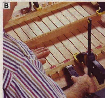
Apply light clamp pressure to the cauls. Use a pry bar to push the cladding against end spacers. Tighten the clamps.
